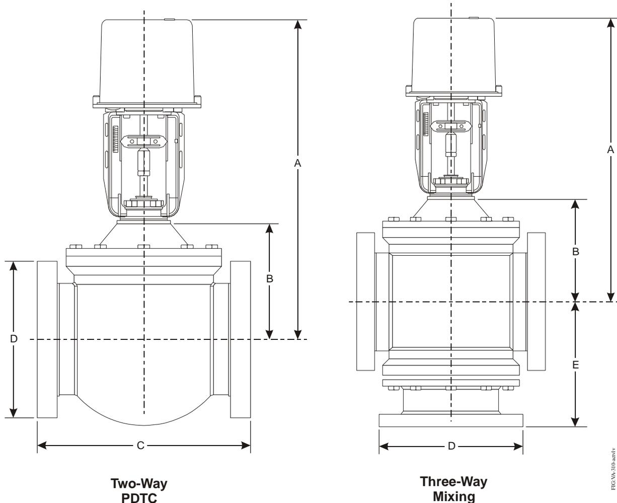
**Figure 5: VA-310x Actuated Valve Dimensions
