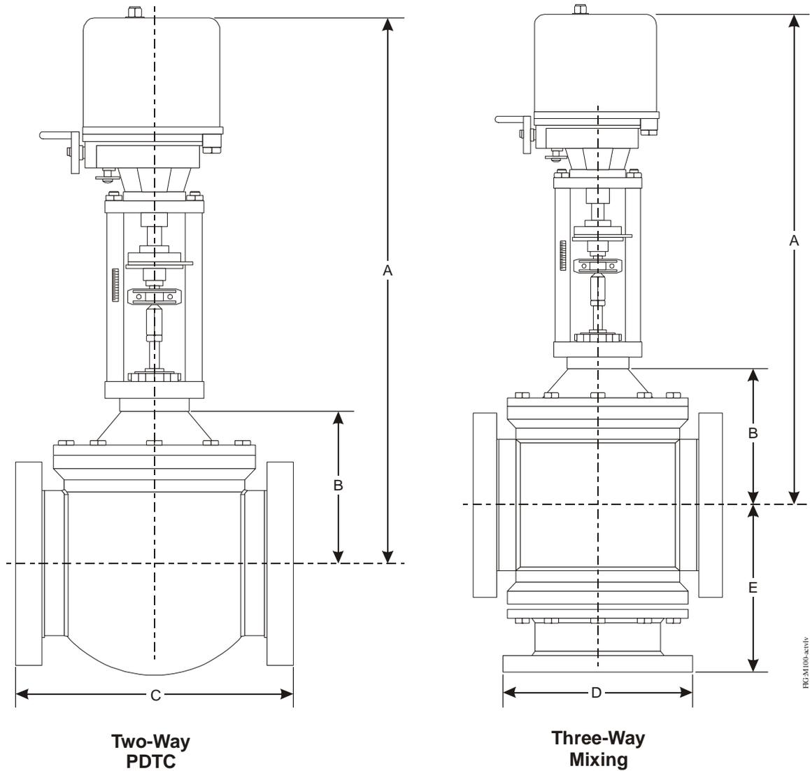
**Figure 6: VA-610x Actuated Valve Dimensions
