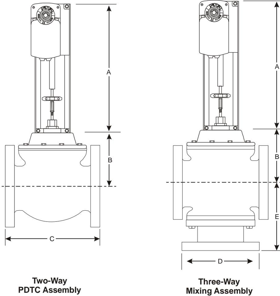
**Figure 4: M9000 Actuated Valve Dimensions, in. (mm)
