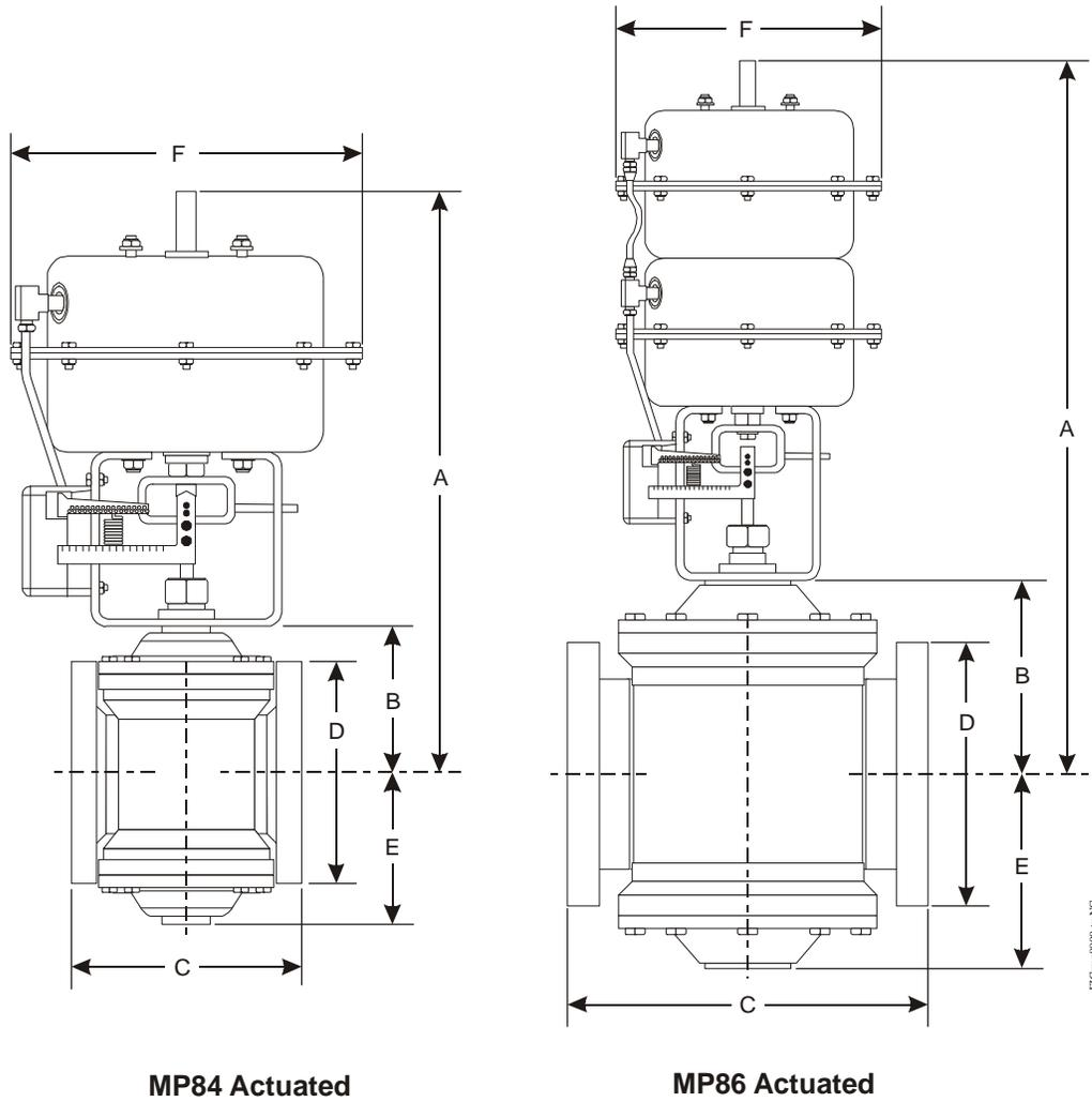
**Figure 2: MP8000 Actuated Two-Way N.C. Valve Dimensions
