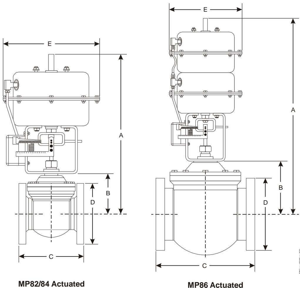
**Figure 1: Dimensions for MP8000 Actuated Two-Way N.O. Valve
