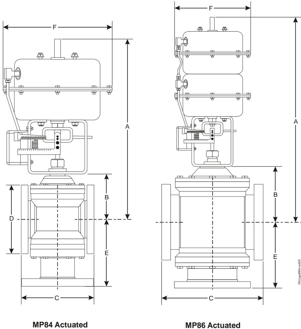
**Figure 3: MP8000 Actuated Three-Way Mixing Valve Dimensions
