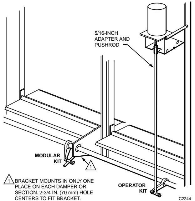
**Fig. 25. Normally open damper jackshaft installation.**
