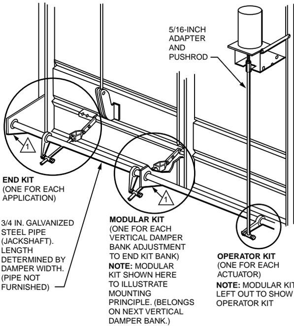
1 BRACKET MOUNTS IN ONLY ONE PLACE ON EACH DAMPER OR SECTION. 2-3/4 IN. (70 mm) HOLE CENTERS TO FIT BRACKET. C2243
