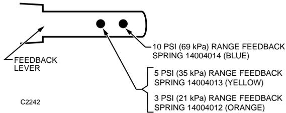
**Fig. 33. Feedback Spring Hook Location.**
