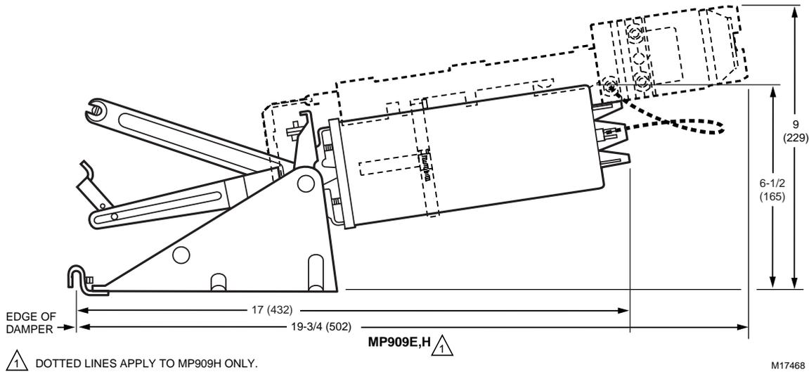
Fig. 13. Internal Mounting Normally Open Dimensions in in. (mm).
