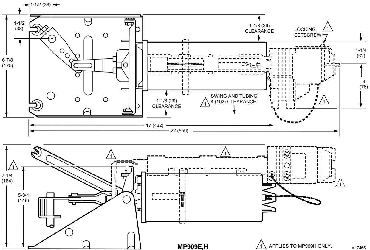
Fig. 7. External Mounting Dimensions in in. (mm) with Trunnion Bracket.
