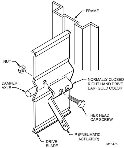
Fig. 2. Normally Closed Drive Ear Mounting.
