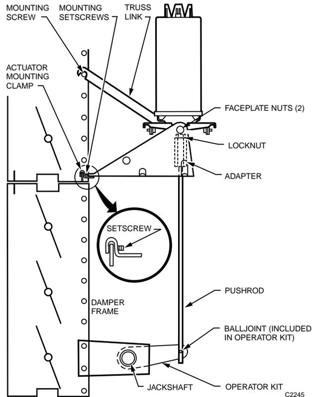
**Fig. 26. Internal Mounting on Damper Frame.**
