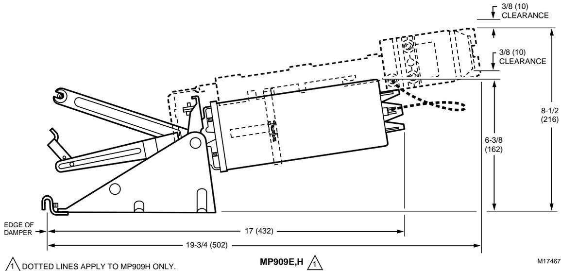
Fig. 11. Internal Mounting Normally Closed Dimensions in in. (mm).
