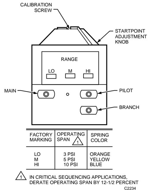
Fig. 32. Original Feedback Spring Marking.
