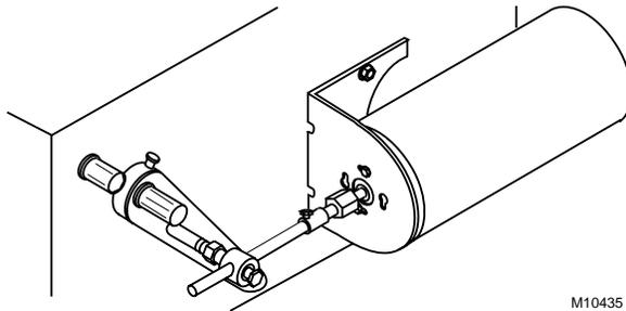
Fig. 6. External Mounting with Angle Bracket.
