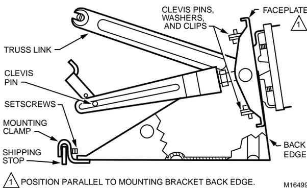
Fig. 12. Internal Mounting Normally Open Faceplate.
