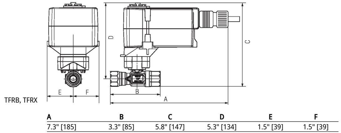
On/Off, Floating point, Non fail-safe, 24 V
