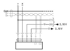
MP-Bus, supply via 3-wire connection
