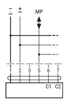
MP-Bus via 2-wire connection, local power supply
