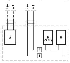
A = Actuator H [% RH] = Humidistat H = Heating
