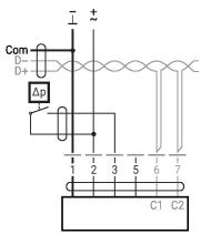
Switching contact requirements: The switching contact must be able to switch a current of 16 mA at 24 V accurately.
