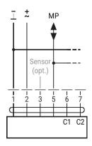
Examples of external wiring with actuator types ..24GX..
