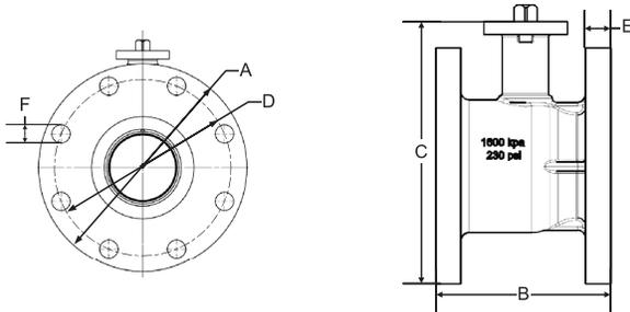
NOTES: Flange bolt pattern with dimensions according to ASME Class 250
