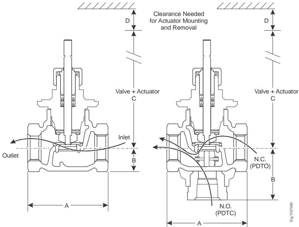
**Figure 2: Two-Way Normally Open (N.O.)/Push-Down-to-Close (PDTC), Two-Way Normally Closed (N.C.)/Push-Down-to-Open (PDTO), and Three-Way Mixing Valve Dimensions, Fluid Flow Directions, and Port Designations (See Table 1 and Table 2.)**
