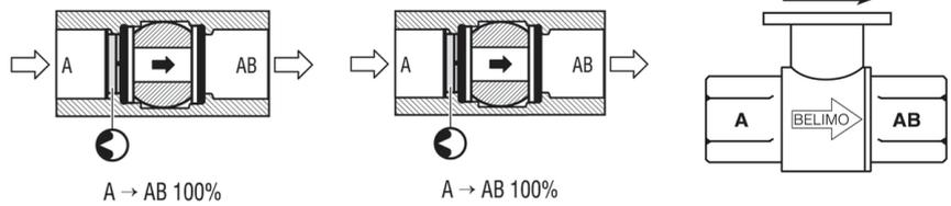
Two-way valves should be installed with the disc upstream.
